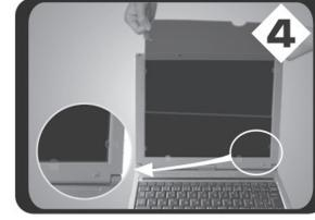
(UK) Insert Secret between the accessory plastic holders and the LCD screen. For indoor use, please place the more reflective surface facing outwards. For outdoor use, use the opposite side, to make for an adjustment to the different light conditions in an outdoor environment.
