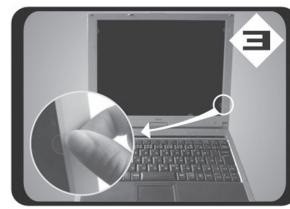
(UK) Paste the adhesive side of the accessory plastic holders at the frame edge of the LCD screen.
